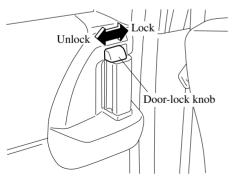
To lock a sliding door with the door-lock knob from the outside, slide the door-lock knob toward the front to the lock position and close the door (pulling the door handle is not required).
